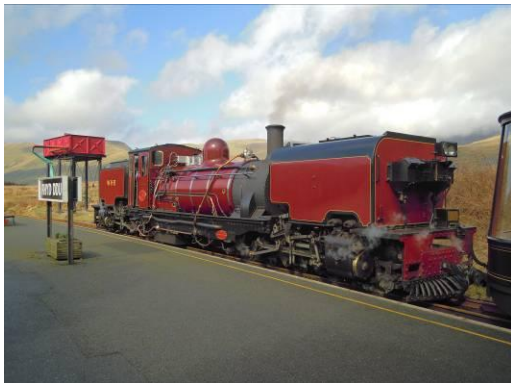
The locomotives are Beyer-Garret articulated steam engines, one built in Belgium for South African Railways and the other at Boston Lodge works. The two trains pass each other at Rhyd Ddu below Snowdon, and it is just as open, empty and bleak as in 1920s photos.
