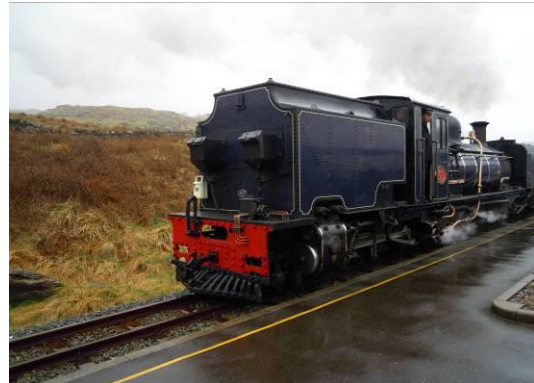
The locomotives are Beyer-Garret articulated steam engines, one built in Belgium for South African Railways and the other at Boston Lodge works. The two trains pass each other at Rhyd Ddu below Snowdon, and it is just as open, empty and bleak as in 1920s photos.
