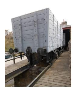
Restored chaldron waggons on the coal staithes. The long levers on either side open the waggon bottom to drop coal into the yard below.
