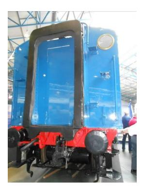
No 4468 Sir Nigel Gresley. The side flaps which originally covered the motion were later removed from all the locomotives. A rear view shows the corridor connection through the tender. By allowing a crew change to take place while on the move, the locos could run the 400 miles nonstop. The drivers and firemen must have been very slim!
